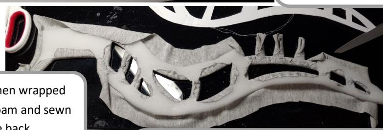
The knit is then wrapped around the foam and sewn to the back
